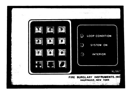
The Model XL567 Digital Key Remote is designed to arm/disarm and bypass control panels in the XL1215 series, utilizing two separate four digit field programmable codes. The code must be entered in sequence. If a wrong digit, or digit out of sequence is pressed, the code must be re-entered from the first digit. Any digits entered will be kept in memory, as long as power is not interrupted.
